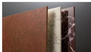
Noncombustible panel for wall whose main constituents are inorganic raw materials. They include wall finishing materials made by decorating calcium silicate boards with resin or sheets, extruded cement panels for exterior walls, and interior wall materials with humidity regulation and deodorant properties.
